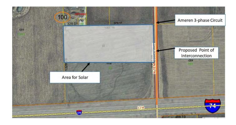
The request is for 3-phase 12kV information on the Ameren distribution circuit on Tennessee Ave on the east side of the property. The proposed point of interconnection is a line tap approximately at the marked point of interconnection.
